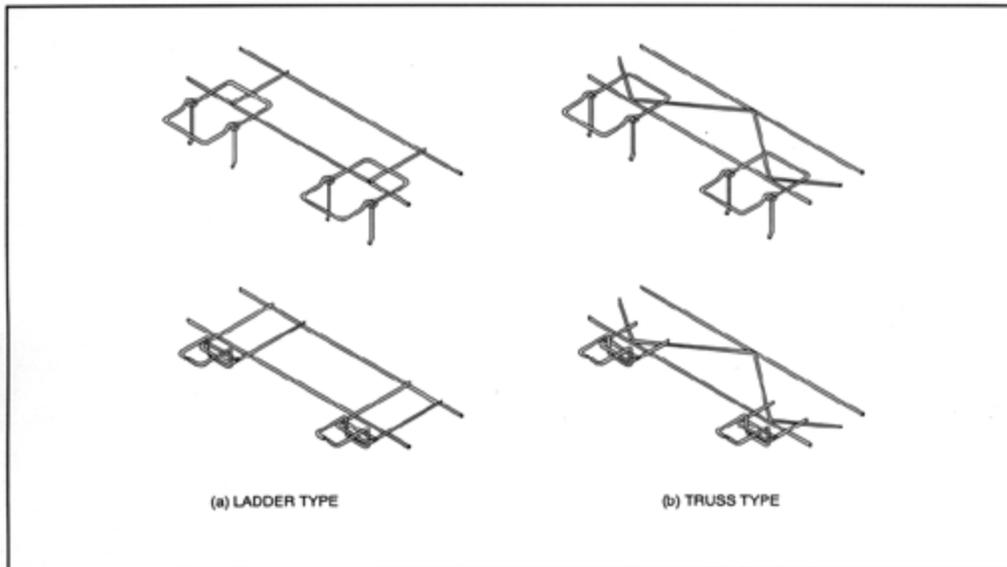
**Adjustable Joint Reinforcement**
